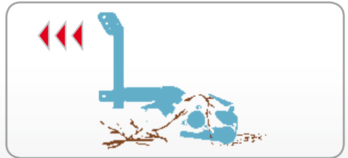
Closed rear hood: to finely mulch prunings and branches
